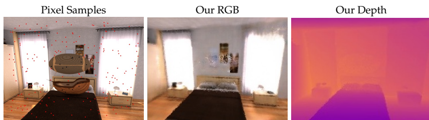
Figure 5.8: Robustness to Dynamic Objects. We show the sampled pixels overlaid on an image with a dynamic object in the center (left), our rendered RGB (middle) and our rendered depth (right) to illustrate the ability of handling dynamic environments. The masked pixel samples during tracking are colored in black, while the used ones are shown in red.
