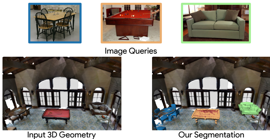
Figure 6.11: Image-based 3D Object Detection. A 3D scene (bottom left) can be queried with images from Internet (top) to find matching 3D points (bottom right). The colors of the image query outlines indicate the corresponding matches in the 3D point cloud. All 3 images are under Creative Commons licenses.
